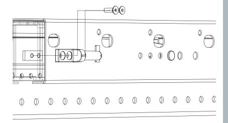
Hinge pin with catch nose and without catch nose
