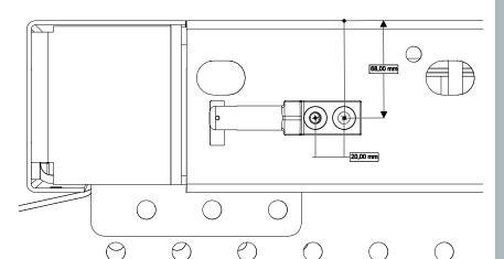
Hinge pin with catch nose and without catch
