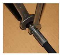
For mounting the hose the open-end wrench sizes **22** and **14** are needed.
