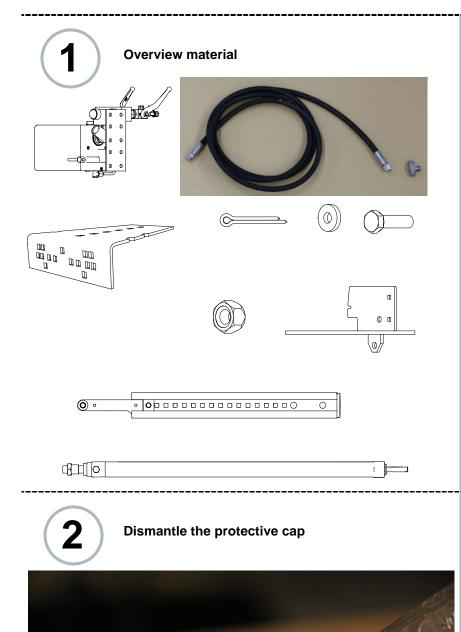
Hoses, connectors and hydraulic cylinders have tob e taken from the **applicable assembly kit.**
