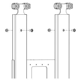
The screws at the upper end of the guide carriages must be removed.
