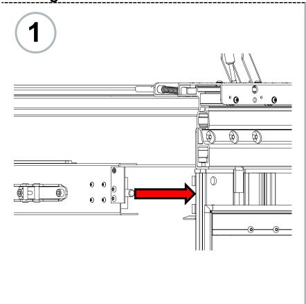
Swivel the lower crossbeam into the direction of the arrow and let it snap in.
