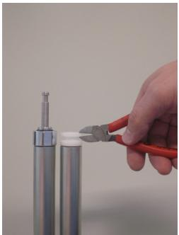
After mounting the compact hydraulics, the tank cap must be cut open for ventilation and air exhaust.
