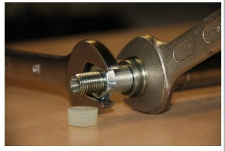
Remove the protective cap and then loosen the nut.
