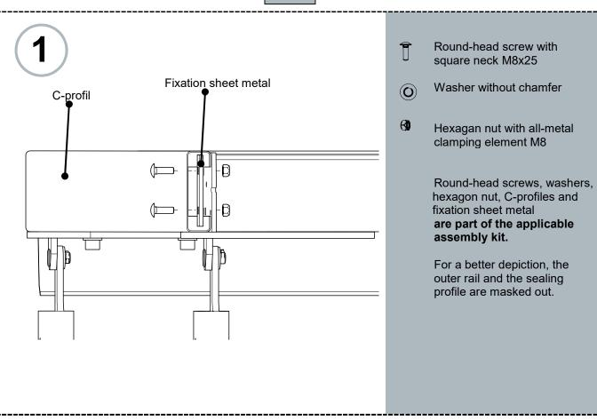
Mounting of sealing sheet metal (only for tops with lifting device)
