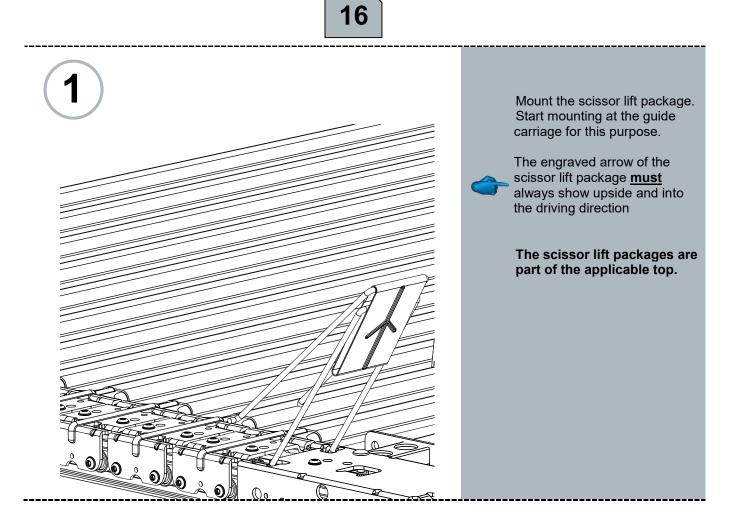
Mounting of adjustment guide carriage backside
