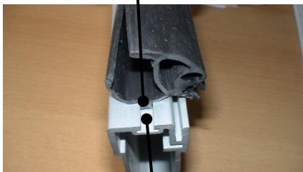
Use lubricant in the T-slot
